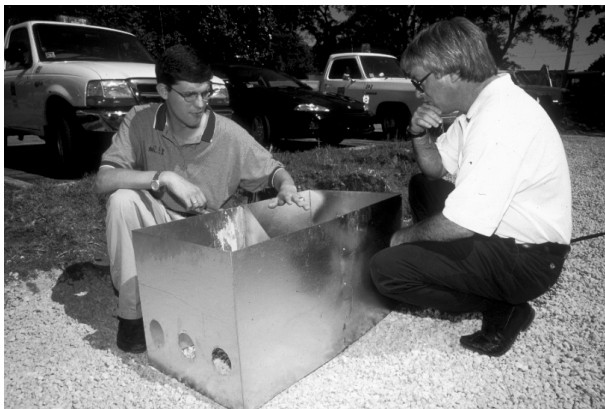
Figure 5. Weir box before installation. Note three holes which allow water to enter from the bottom, establishing a still area into which a flume stick can be installed. The presenter's hand is directly over the v-notch weir.
