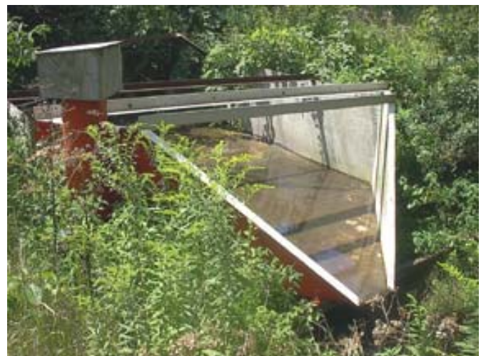
Figure 3. HL-flume at the Finley West paired-watershed monitoring site.
