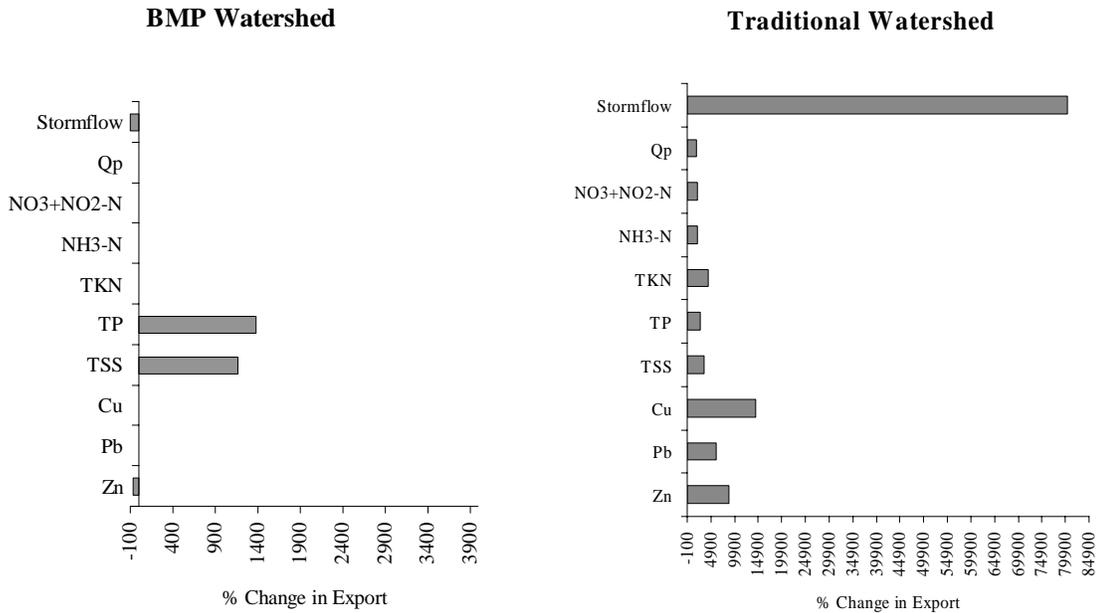
**Figure 7. CONSTRUCTION PERIOD RESULTS** for the BMP and traditional watersheds. Bars represent the percent change observed due to construction that is calculated from the difference between the observed value and the value predicted by the calibration regression equation. Bars are not shown for non-significant differences.
