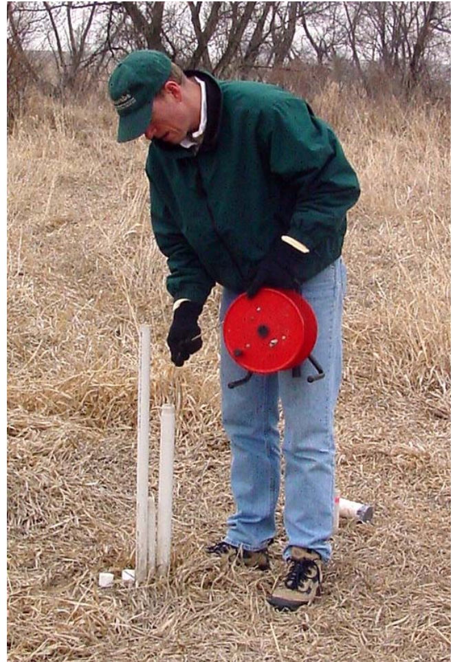
Figure 3. Monitoring wells have been installed at the refuge to track changes in groundwater quality over time.
