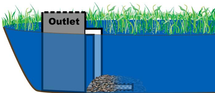
Figure 8: Illustration of a possible modified outlet structure for temperature reduction.
