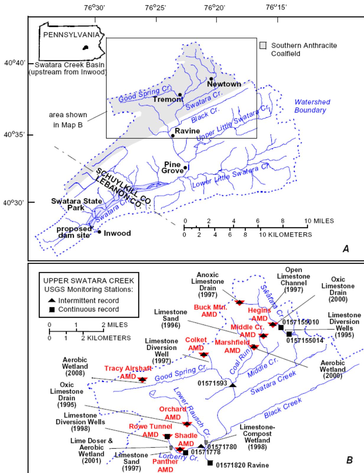
**Figure 1.** Municipalities, “acidic” mine drainage (AMD), AMD treatment with year of implementation in parentheses, and USGS monitoring stations in the Swatara Creek Basin upstream from the proposed dam for Swatara State Park Reservoir, Lebanon and Schuylkill Counties, Pennsylvania. USGS monitoring station numbers are indicated for sites with fish data.
