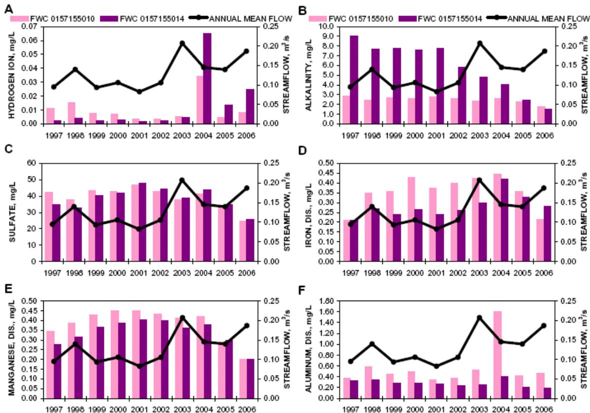
**Figure 13.** Annual mean streamflow for Swatara Creek at Newtown (0157155014; black bar) and corresponding flow-weighted concentration (FWC) of chemicals upstream (0157155010; left bar) and downstream (0157155014; right bar) of diversion wells, 1997-2006: A, hydrogen ion; B, alkalinity; C, sulfate; D, dissolved iron; E, dissolved manganese; F, dissolved aluminum.
