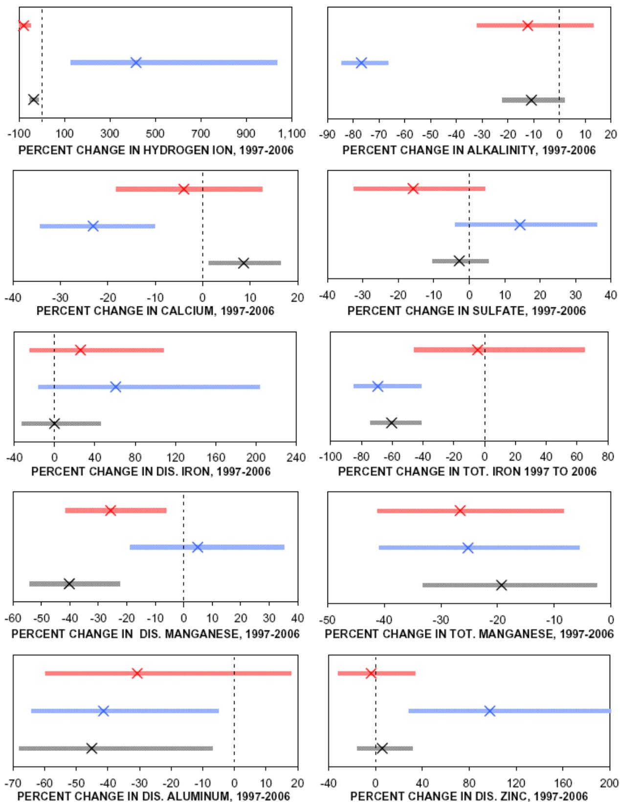
**Figure 14.** Estimated flow-adjusted trend (X) and confidence interval (CI) bar for chemicals in Swatara Creek at Ravine (01571820; lower black bar) and Swatara Creek at Newtown downstream (0157155014; middle blue bar) and upstream from diversion wells (0157155010; upper red bar), 1997-2006. If the CI is completely negative or completely positive, the trend is significant.
