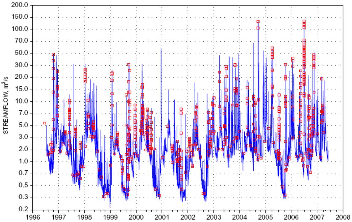
**Figure 7.** Streamflow hydrograph (recorded at 15-minute intervals) for Swatara Creek at Ravine, Pa., June 1996 through June 2007. Square symbols indicate instantaneous streamflow when water-quality samples were collected.
