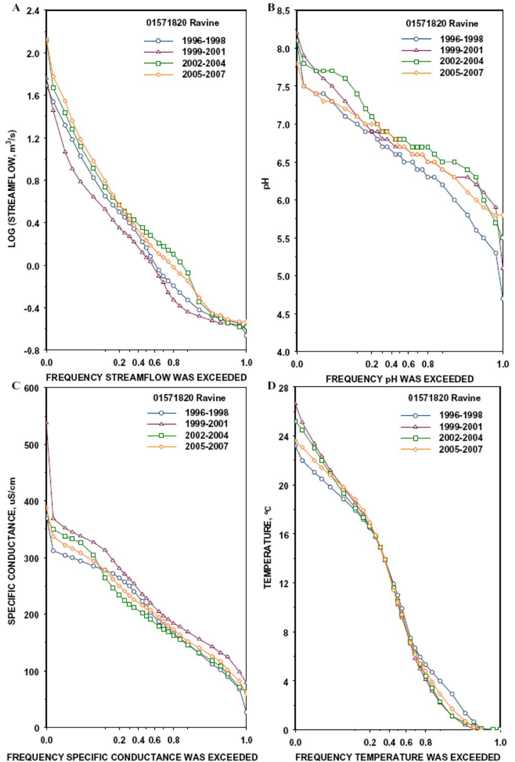
**Figure 4.** Probability plots of continuously measured (recorded at 15-minute intervals) data for Swatara Creek at Ravine, Pa., September 1996 through September 2007: A, streamflow; B, pH; C, specific conductance; D, temperature. The X-axis indicates the frequency that values were exceeded during 3-year intervals.
