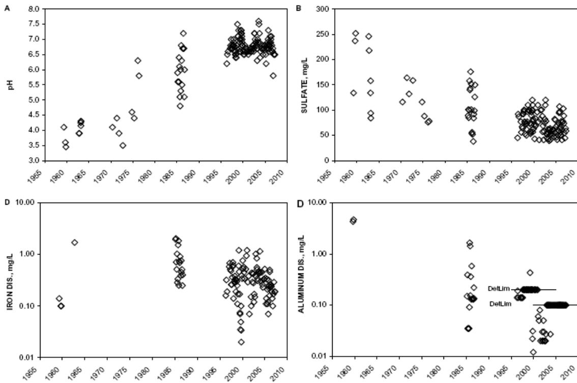
**Figure 8.** Long-term water-quality data for base flow of Swatara Creek at Ravine, 1959 - 2007: A, pH; B, dissolved sulfate; C, dissolved iron; D, dissolved aluminum. Data from McCarren et al. (1964), Stuart et al. (1967), Skelly & Loy, Inc. (1987), Fishel (1988), and U.S. Geological Survey (variously dated). Aluminum concentrations below detection are shown at detection limit (DetLim), indicated by horizontal line segments.
