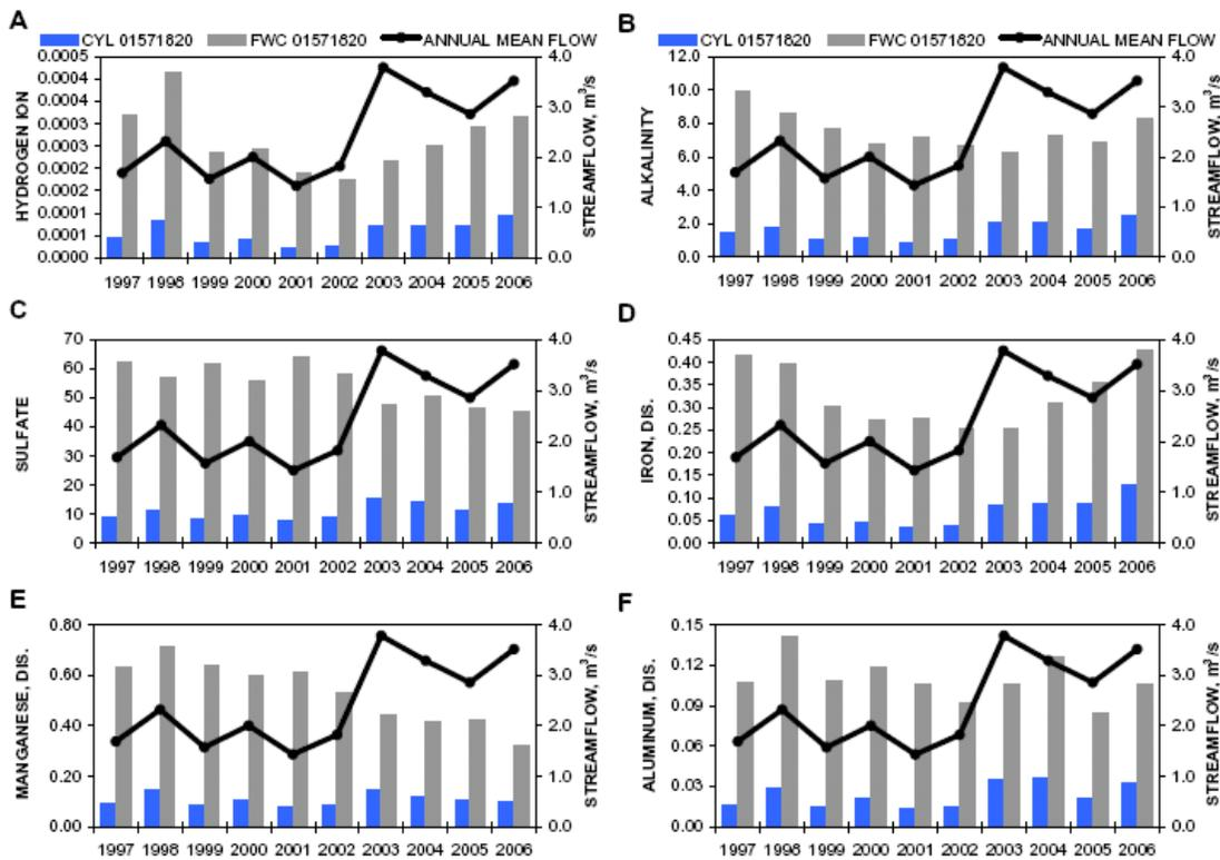
**Figure 12.** Annual mean streamflow for Swatara Creek at Ravine (01571820; black line) and corresponding loading by calendar year (CYL; left bar, units Mg/day) and flow-weighted concentration (FWC; right bar, units mg/L) of chemicals associated with mine effluent, 1997-2006: A, hydrogen ion; B, alkalinity; C, sulfate; D, dissolved iron; E, dissolved manganese; F, dissolved aluminum.
