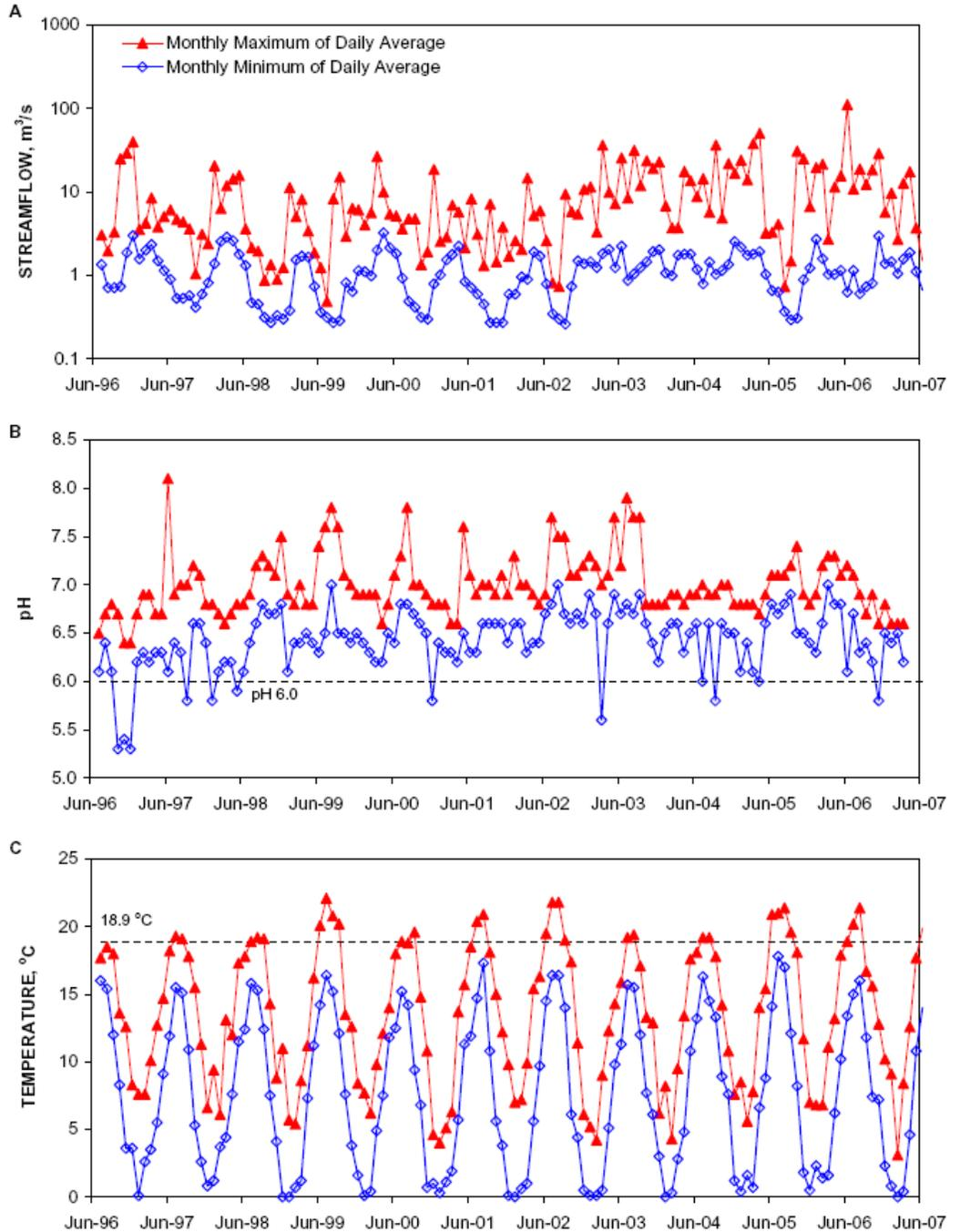
**Figure 5.** Time-series plots of the monthly range (maximum and minimum) of daily mean values for Swatara Creek at Ravine, Pa., June 1996 through June 2007: A, streamflow; B, pH; and C, temperature. In B and C, dashed horizontal lines indicate minimum pH and maximum temperature permitted for “cold-water fishery” in July and August, respectively (Commonwealth of Pennsylvania 2002).
