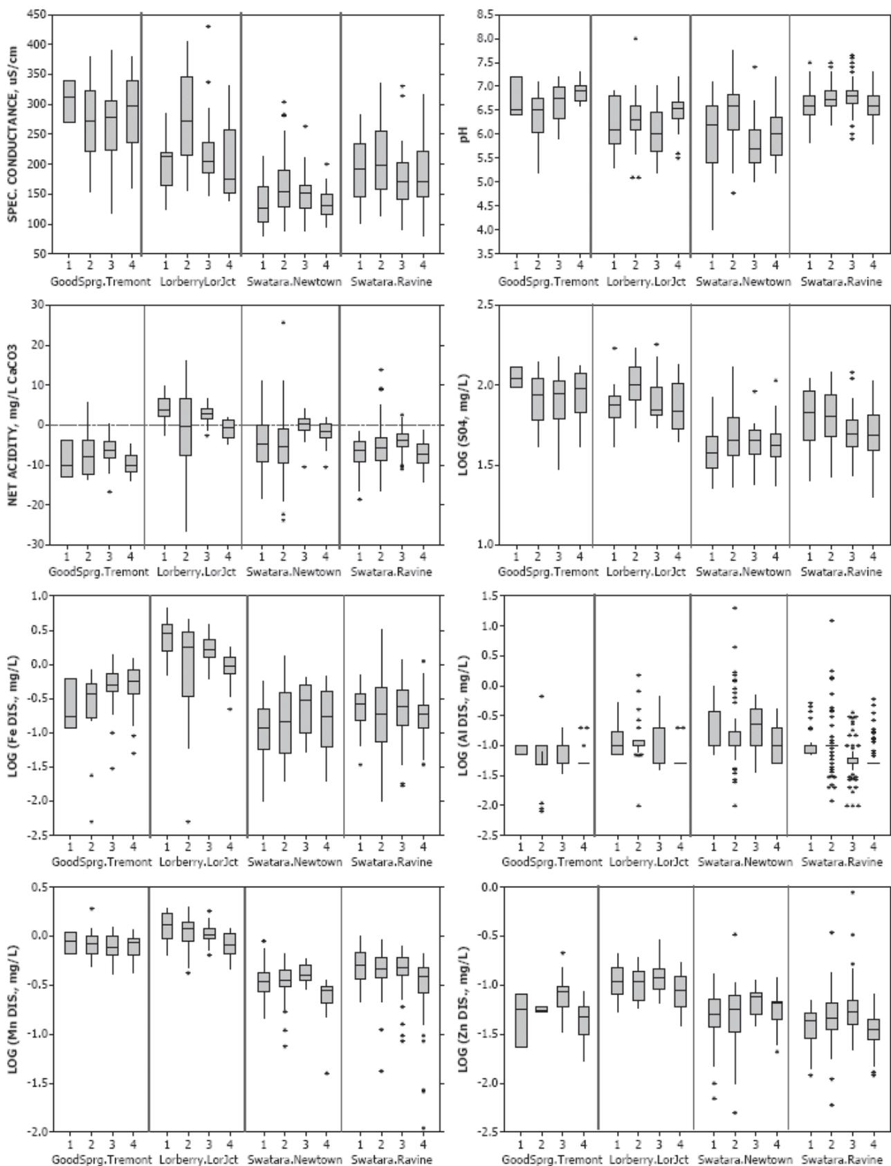
**Figure 3.** Boxplots summarizing hydrochemical characteristics of stream water at sites of annual fish surveys in Swatara Creek Basin, Pa., over 3-year intervals: (1) 1996-1998, (2) 1999-2001, (3) 2002-2004, (4) 2005-2007. Shaded area of box indicates the “interquartile” range (IQR = 25th to 75th percentile); horizontal line inside the box indicates the median; vertical lines extend to extreme values within 1.5 times the IQR; symbols indicate outlier values.
