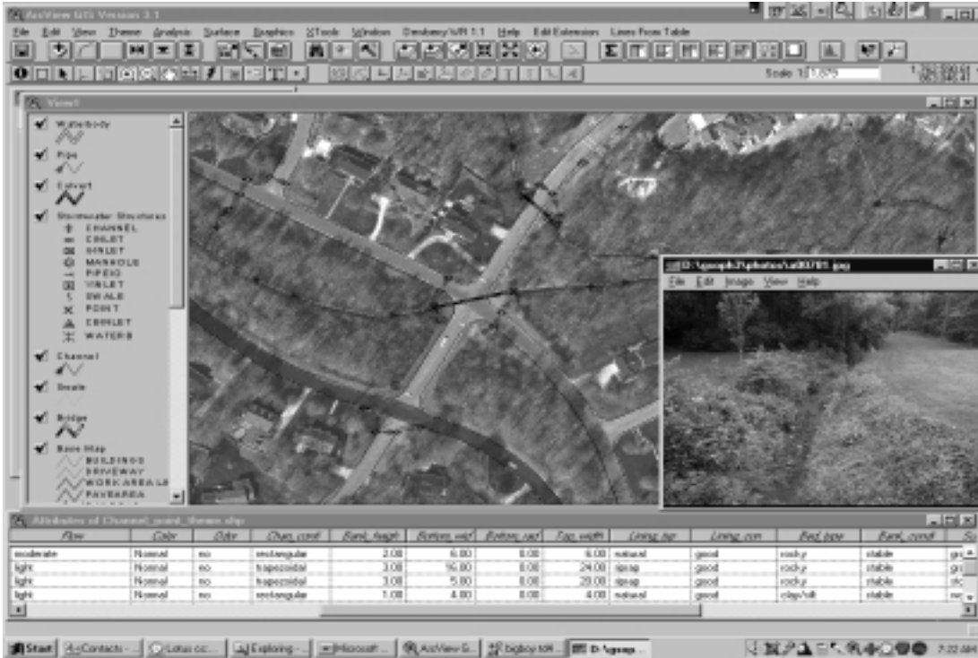
Figure 2. Stormwater system inventory module.
