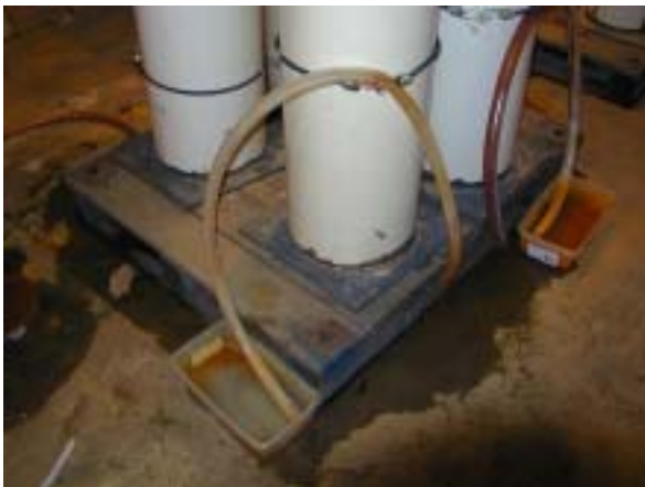
Figure 2. Columns tested at Penn State included the ability to create an anaerobic zone using flexible tubing. Each was filled with four feet of Cecil Sandy Loam.
